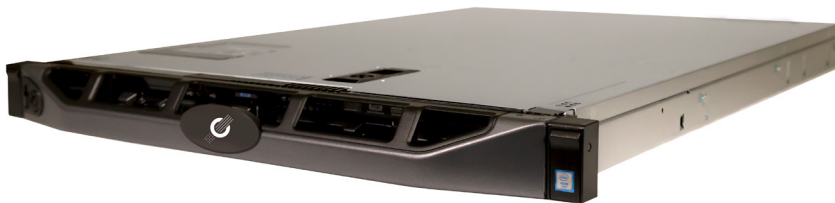
TSF 400: QRNG + Key Manager + HSM integrated into one device
